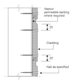
Figure 3 Shiplap or Chamferboard
